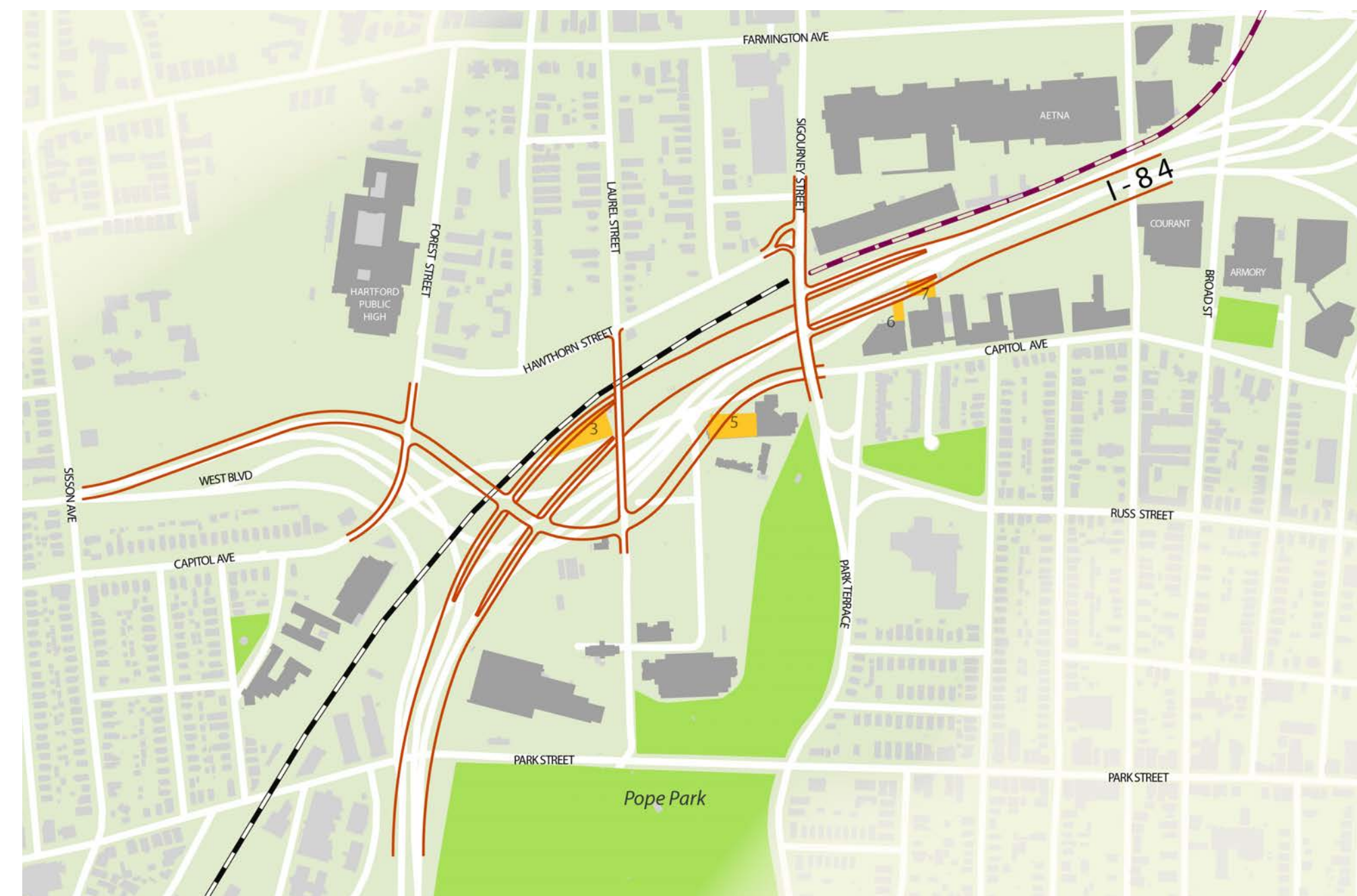
West Boulevard extension to Capitol Avenue Full Diamond Interchange At-Grade Intersections at Forest Street and Laurel Street
