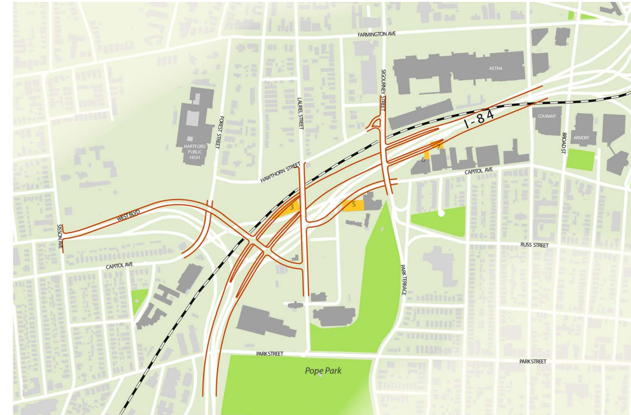
West Boulevard extension to Laurel Street Full Diamond Interchange Capitol Avenue realigned with Forest Street
