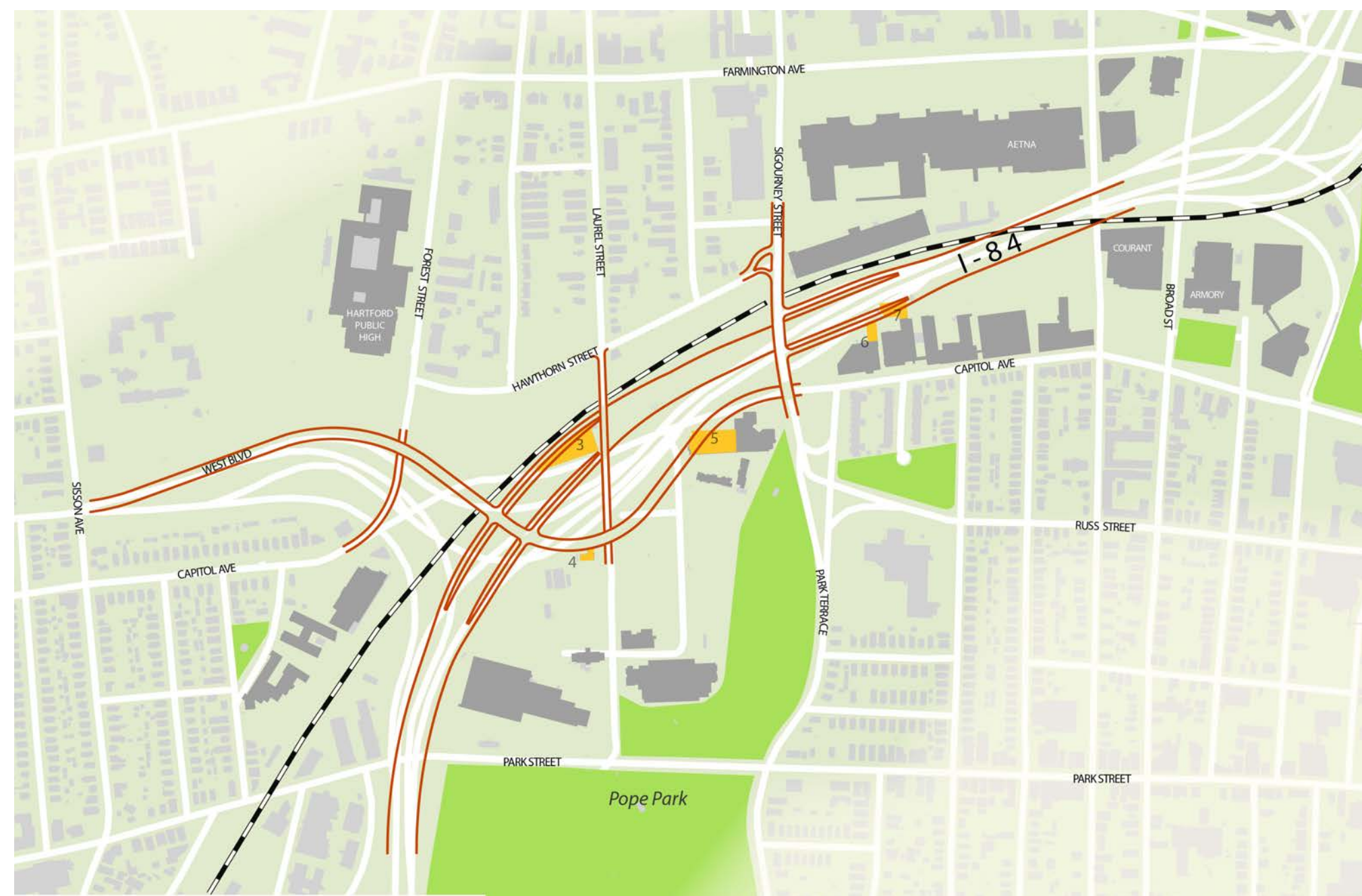
West Boulevard extension to Capitol Avenue Full Diamond Interchange Grade-Separate Intersections at Forest Street and Laurel Street
